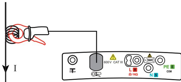
Here, the conductor passes through the clamp 4 times. You will have to divide the measured current by 4 to know the true value of I.
