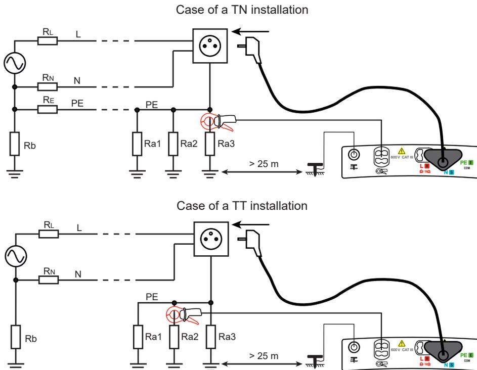
For a more accurate measurement, you can choose a high current (TRIP mode), but the RCD that protects the installation may trip.
