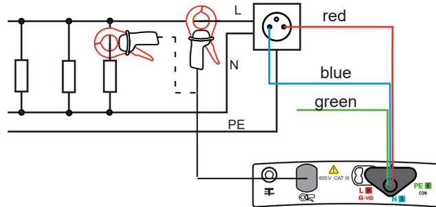
In the case of a three-phase network balanced in voltage and in current, connect the measuring cable terminated by 3 leads to the device and to two of the three voltages  $U_{12}$ ,  $U_{23}$  or  $U_{31}$  using the red and blue leads. Then, with the clamp, surround the conductor of the third phase  $I_3$  (for  $U_{12}$ ),  $I_1$  (for  $U_{23}$ ) or  $I_2$  (for  $U_{31}$ ).
