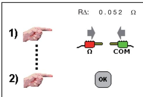
Connect the two leads that you are going to use for the measurement to the  $\Omega$  and COM terminals, short-circuit them, then press the **TEST** button.
