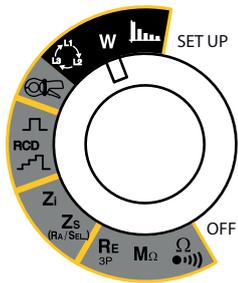
In the case of a single-phase network, connect the measuring cable terminated by 3 leads to the device and to a socket outlet of the installation to be tested, using the red and blue leads. With the clamp, surround either the phase conductor, to obtain the total power, or the conductor of one of the loads, to obtain the partial power.
