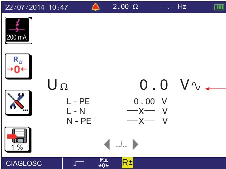
External voltage present on the terminals just before the start of the measurement.
