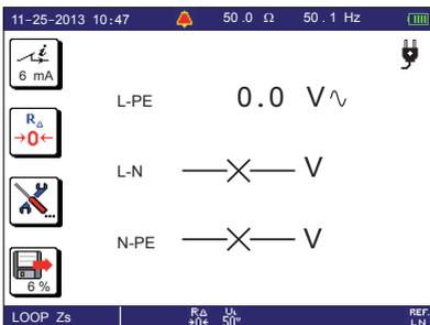
If  $U_{N-PE}$  does not display – x –, the protection in the N terminal has been activated.
