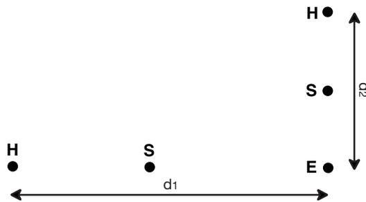
If you find the same values, your measurement is reliable. If the measured values are substantially different, it is probable that they were influenced by earth currents or a groundwater artery. It may be useful to drive the rods deeper.
