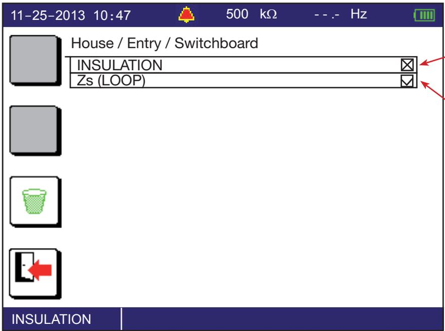
Insulation resistance measurements have been made on this OBJECT and at least one of them is not OK.
