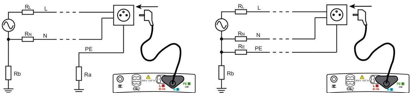
**i** In trip mode, it is not necessary to connect the N terminal.
