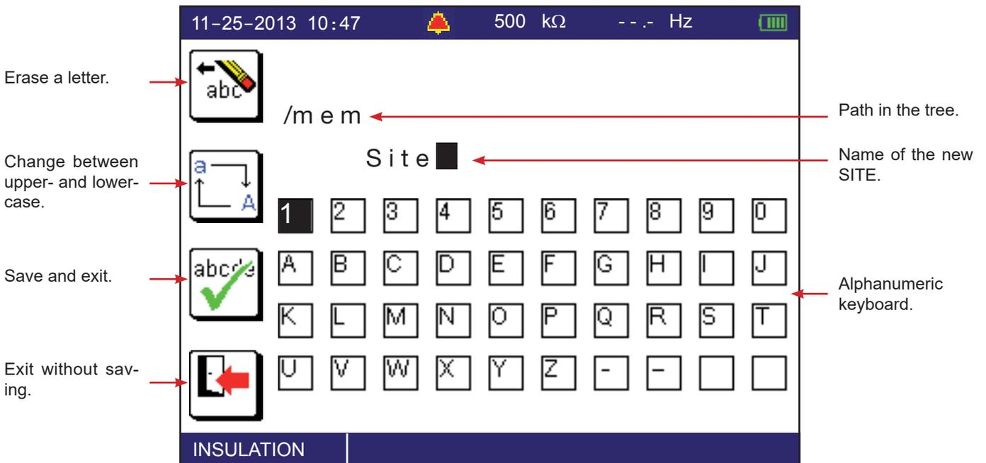
You can then rename the SITE. Start by erasing the existing text. Then move about on the keyboard using the directional keypad (▲▼◀▶) and validate each letter by pressing the OK key.
