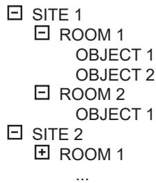
Each OBJECT can contain 9 tests of each type (insulation, earth measurement, RCD test, etc.).
