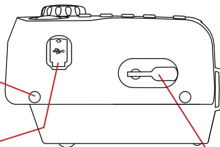
Fasteners for the hand strap, also used to tilt the device.
