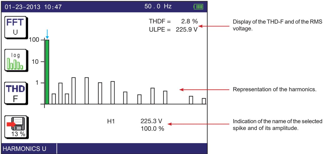
The frequency and amplitude of the selected harmonic (in green) are indicated at the bottom of the graph. To select another harmonic, use the ◀ ▶ keys. The device then shifts from the fundamental (H1) to harmonic H2, then to harmonics (H3, H4, ..., H25). And on the next page it sweeps the harmonics from H26 to H50.
