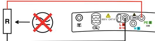
To avoid leakage during the insulation measurement, which would throw off the measurement, **do not use** the measuring cable when you make this type of measurement, but two simple leads.
