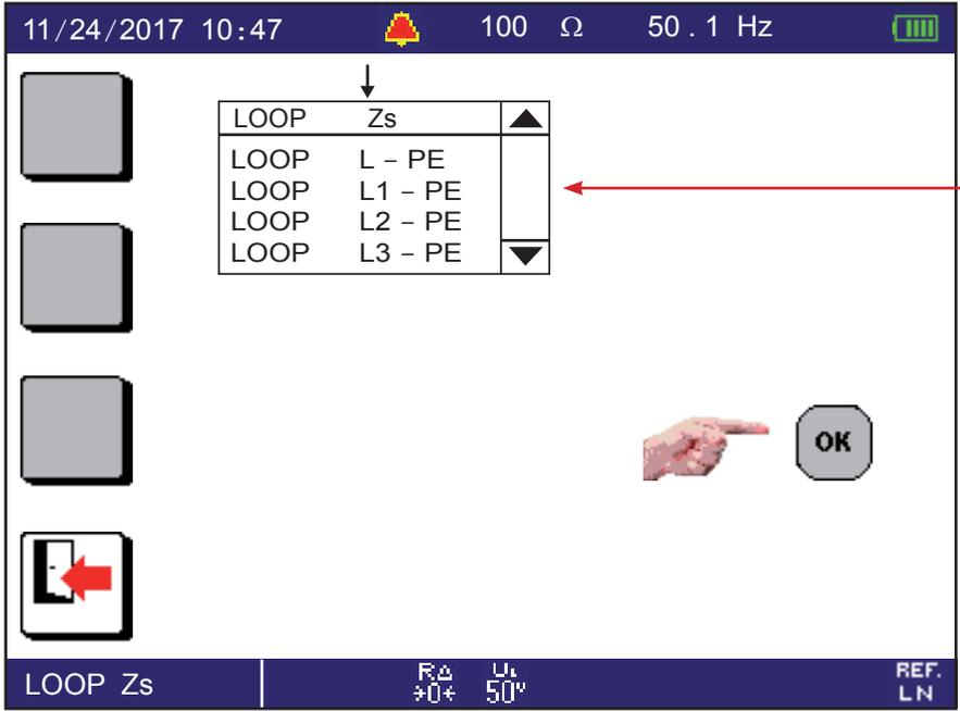
As in the case of insulation, you can index the measurement.
