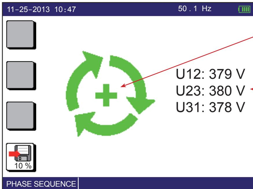
The + sign indicates a forward direction and the - sign a reverse direction.
