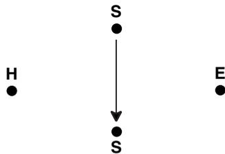
Avoid routing the connecting cables of the earth rods near or parallel to other cables (transmission or power supply), metal pipes, rails, or fences, this in order to avoid the risk of cross-talk with the measurement current.
