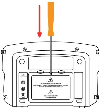
2. Turn the device over and insert a screwdriver into the hole in the battery pack.
