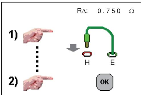
Connect the lead that you are going to use to connect the E terminal to the earth between the H and E terminals, then press the **TEST** button.
