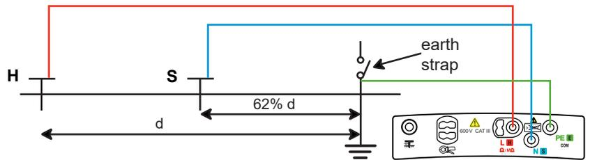
Connect the cables to the H and S terminals. Power down the installation and disconnect the earth strap. Then connect the E terminal to the earth electrode to be checked.
