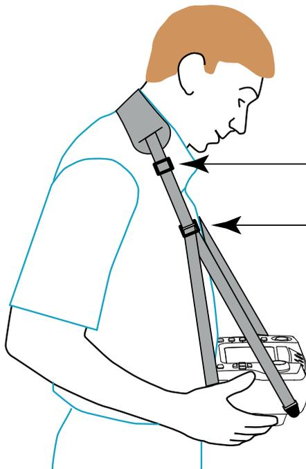
The 4-point hands-free strap will let you use the device while leaving your hands free. Snap the four fasteners of the strap onto the four lugs on the device.
