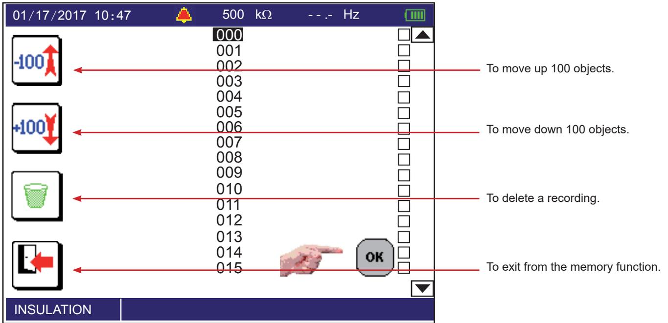
Use the ▲▼ arrows to select the object in which you want to record your measurement and validate by pressing the **OK** key.
