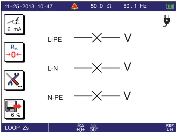
If  $U_{L-PE}$  does not display – x –, the protection in the L terminal has been activated.
