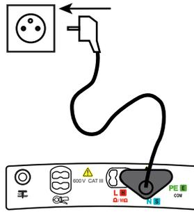
In the  $Z_S$  (RA/SEL.) and RCD, settings, the device also indicates the position of the phase on the display unit using the
