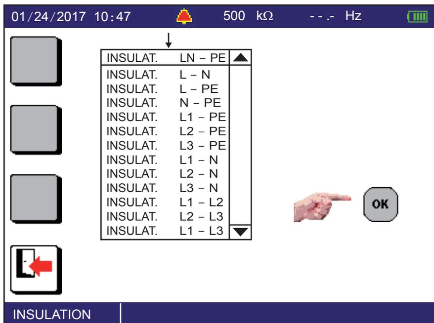
Using the ▲ ▼ arrows, select the type of insulation measurement you have just made and validate by pressing the **OK** key.
