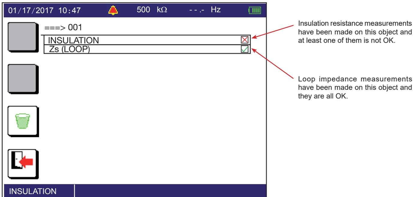
Press the **OK** key to expand one type of test.
