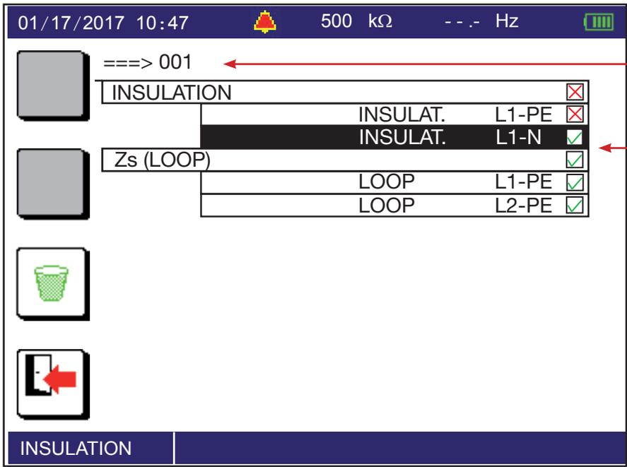
Use the ( ▲▼◀▶ ) keys to select a measurement. Press the **OK** key again to see the recorded measurement.
