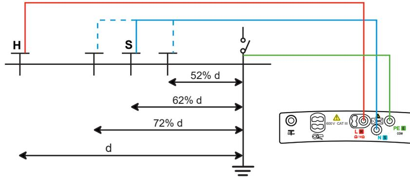
The 3 measurement results must be the same to within a few percent. If this is the case, the measurement is valid. If not, it is because the S rod is in the zone of influence of the earth electrode.
