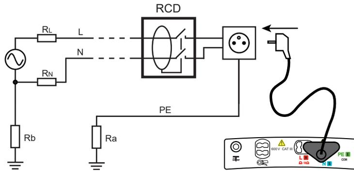
**i** If possible, first disconnect all loads from the network on which you test the RCD. This prevents interference with the test by any leakage currents due to these loads.
